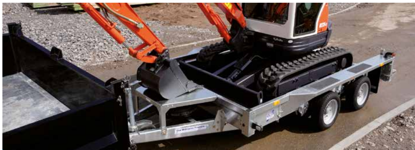
GX106 with skids and integrated rear supports
